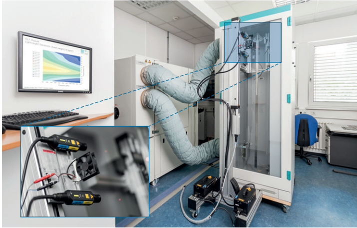
Fig. 30: Test rig for optical loss factor deter- mination according to the OLF Method
