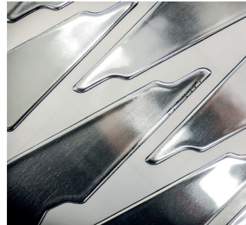
Fig. 23: Aluminum-butyl rubber sandwich system
