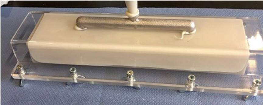
FIGURE 7 Multiple injections with SikaPower Standard (top) and SikaPower SmartFlow (down) (© Sika)
