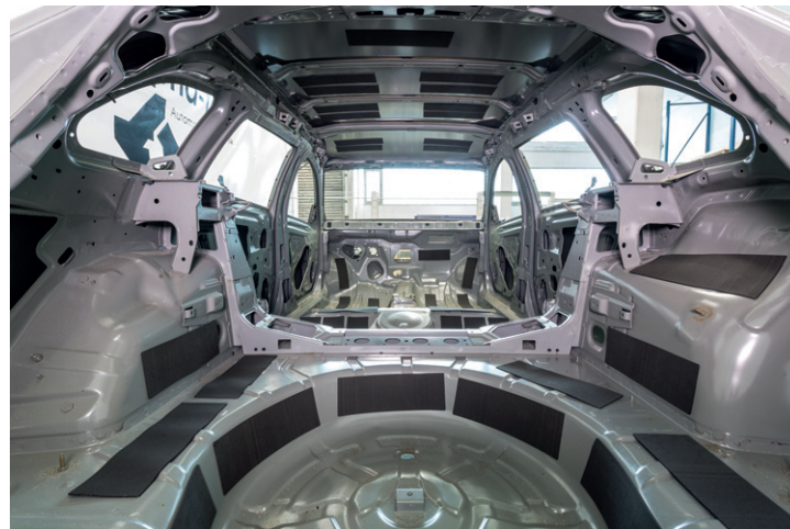
Fig. 15: Damping measures on a body in white: geometric measures and damping coatings are shown.
