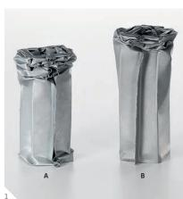
IMPACT TEST RESULTS: (A) Spot welded
