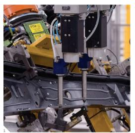
SikaPower® MBX - Central tunnel bonding (CFRP - steel)
