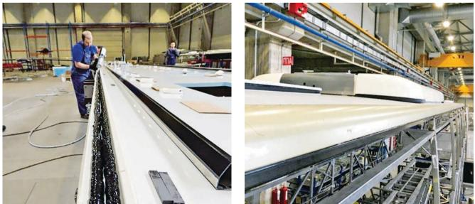
Figure 7 > Application of 'Powerflex' and 'Curing by Design' adhesive for bus roof bonding
