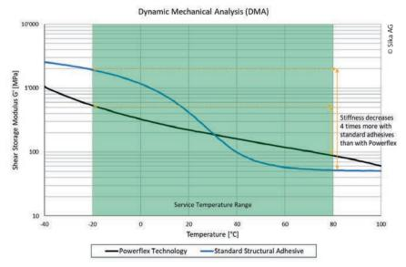
**Figure 1** > Comparison of DMA between "Powerflex" technology and standard structural adhesive in commercial transportation
