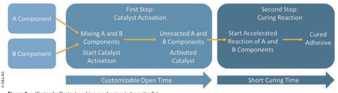
Figure 5 > 'Curing by Design' working mechanism (schematically)
