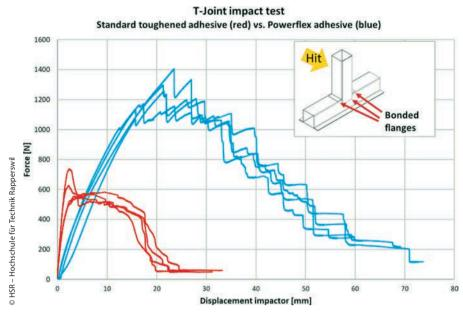
**Figure 3** > Impact tests of T-joints bonded with a standard toughened adhesive (red curves) and a 'Powerflex' adhesive (blue curves): the larger area beneath the blue curves indicate a greater toughness and energy absorption.
