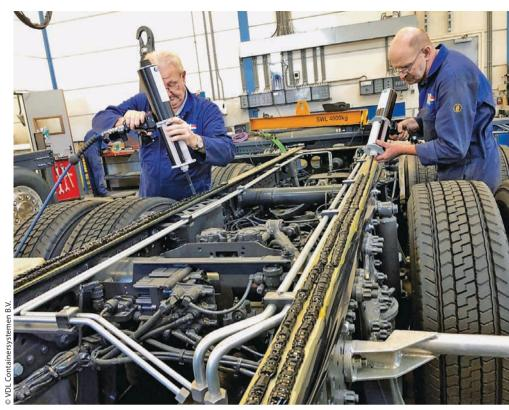
**Figure 6** > Application of 'Powerflex' and 'Curing by Design' adhesive for hook arm bonding on a truck chassis
