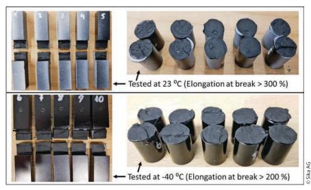
Figure 2 > Cohesive failures of 'Powerflex' adhesive on e-coated steel in 'Thick Adherent Shear Tests' (TAST) and butt joint tensile tests at 23 °C and -40 °C
