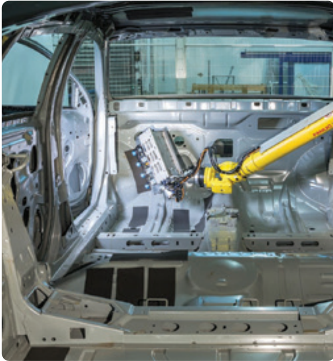
SikaDamp Autopad II enables reliable, repeatable application of damping pads using AI and robotics
