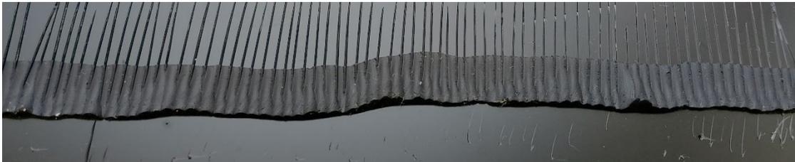
The bead peel test results above (tested before and after common OEM ageing simulations) display fracture patterns demonstrating how stable and reliable adhesion can be obtained with SikaForce®-821 L06 without any physical activation process of the substrates. This offers leaner substrate preparation and bonding processes on important spoiler materials and other components made of PC blends.
