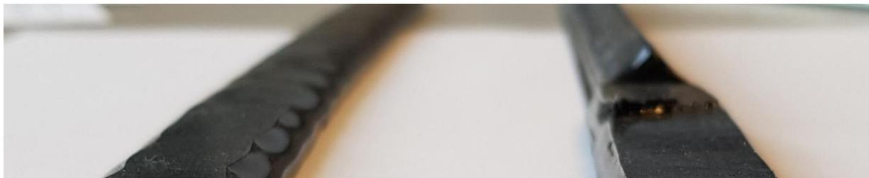
Round and triangle bead could be applied to a compressed bead thickness of 6 mm
