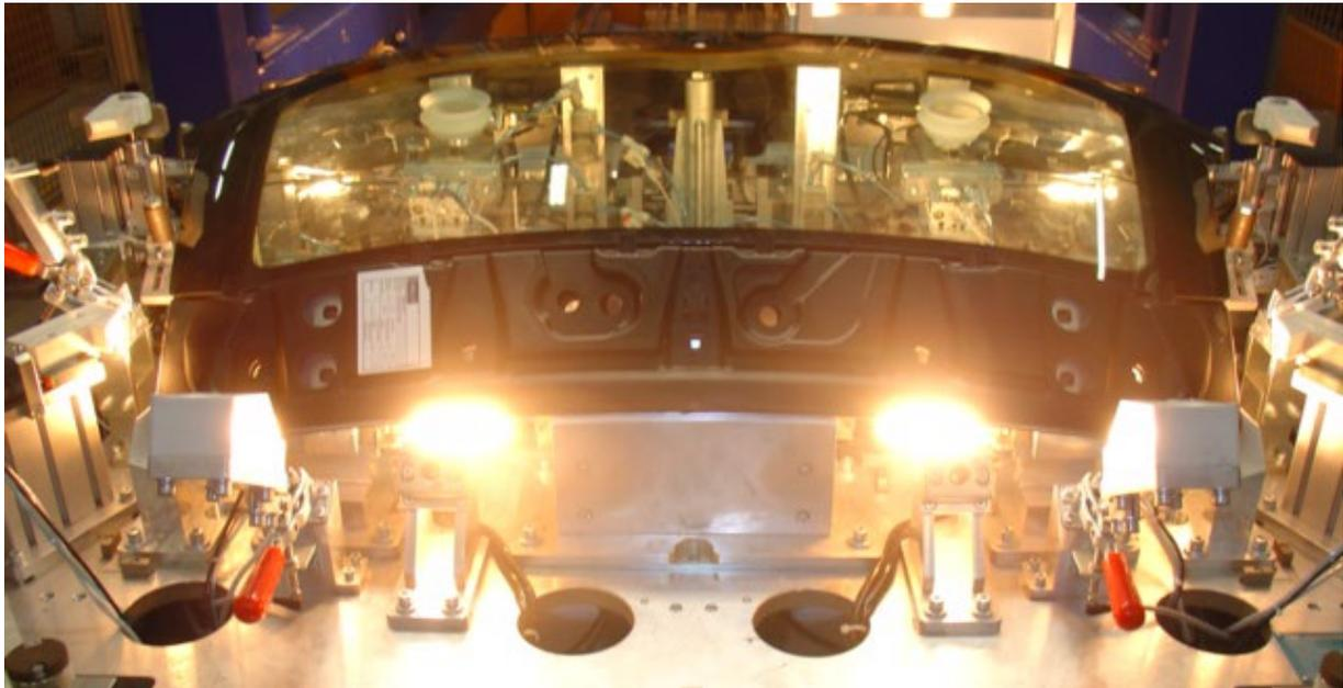
**Figure 1** Typical Curing-On-Demand process with IR radiation
