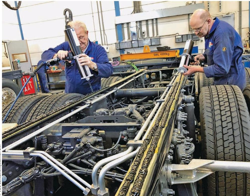
**Figure 6** > Application of 'Powerflex' and 'Curing by Design' adhesive for hook arm bonding on a truck chassis
