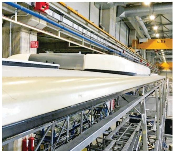
**Figure 7** > Application of 'Powerflex' and 'Curing by Design' adhesive for bus roof bonding
